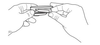
When battery is low, the battery indicator symbol on the display will flash. Remove battery if the device will be stored for more than 30 days. Replace low battery as soon as possible.
